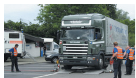
BM20200 used for roadside testing
