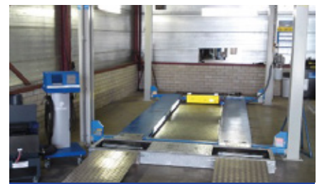
BM3010 roller brake tester on-ground in front of workshop hoist
